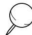
Tack (x2) This is for temporarily holding the bottom row of tiles to the wall during the nailing process.
