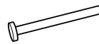
Driver (x2) This is used to drive the nail to the proper depth.
